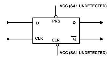
Figure 8: SA1 on both inputs is untestable tied
