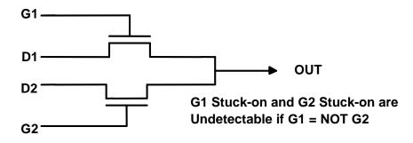
Figure <u>12</u>: <u>Undetectable Fault in a</u> Wired Junction Configuration
