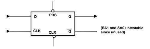
Figure 9: SA1 and SA0 on Q-bar are untestable unused
