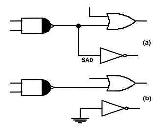
Figure <u>5</u>: (a) Fan-out Logic (b) Same Logic with SA0
