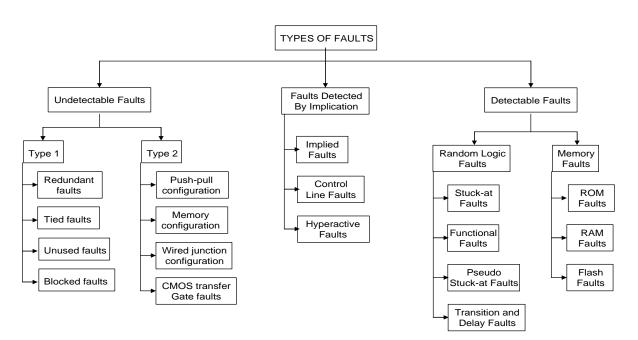
Figure 3: Fault Types
