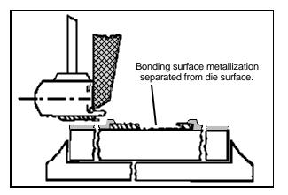
TYPE 6: Bonding Surface Lift
