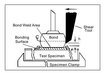
Figure 1: Bond Shear set-up
